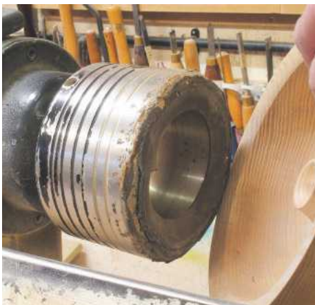
▲ Pic.16 Reversing this bowl is going to be a little more difficult than normal, but the drum chuck off his vacuum system will allow him to cope with the central stem
